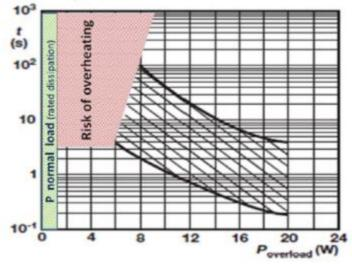
If the fusible resistor is used above the maximum specified overload, there is a risk of explosion. This is due to the fact that there is much more energy available than what the resistor was designed for. The resistor might not be able to dissipate enough energy in a timely manner. This area is represented in the example below:
